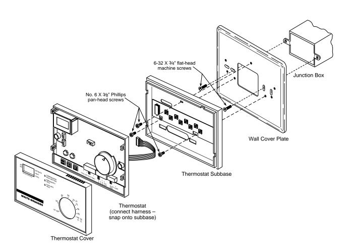
Figure 10. Mounting 1F62 thermostat to horizontal junction box
